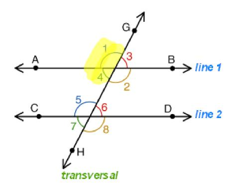
angle  $1 + \text{angle } 3 = 180^{\circ}$ angle  $1 + \text{angle } 4 = 180^{\circ}$
